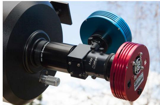
It is probable that the slit direction will have moved : rotate the guiding camera to put it back horizontal. If required, re-focus the slit image in this position.
