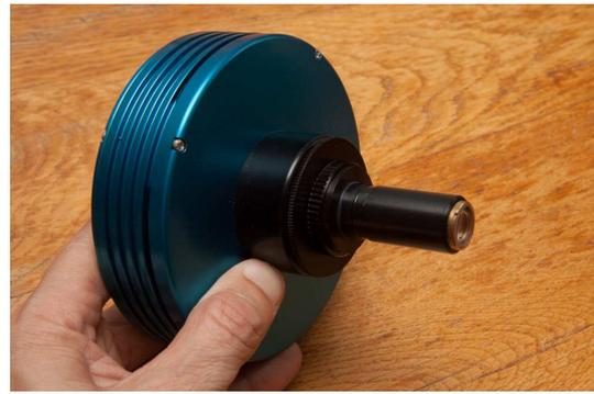
Remove the optics from the guiding module (loosen the two knurled thumb screws):
