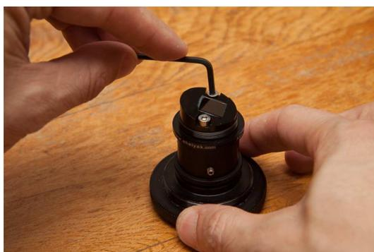
The nominal thickness (base to slit) of the standard and guider slit holders are identical (5mm). However, there is some manufacturing tolerance so you should check that the focus of the Alpy 600 is still correct (refer to the Alpy 600 user guide). From the spectroscopy standpoint, the guided slit is the equivalent of the standard  $25\mu\text{m}$  slit (except the width is  $23\mu\text{m}$  with guiding module).
