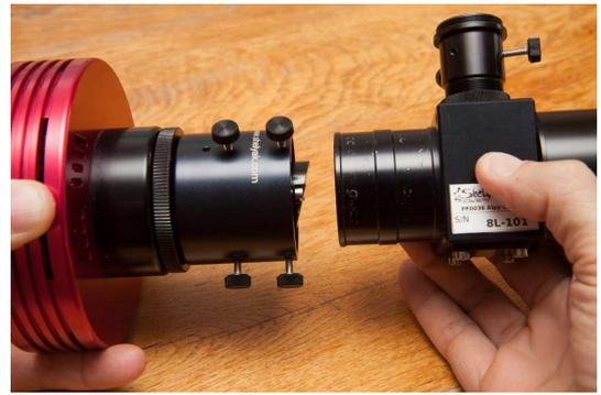
Rotate the spectroscope in such a way that the slit mirror is towards the guiding mirror (in the images below, the 2" adapter has been removed for a better view):
