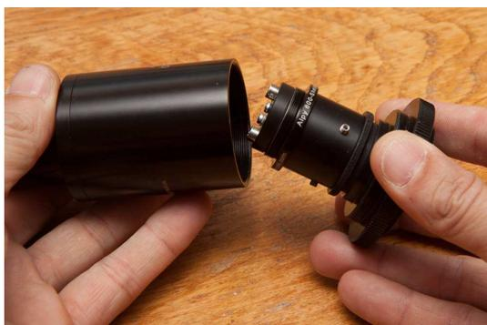
The Alpy 600 spectroscopy has a removable slit holder. Remove the two screws, then the holder:
