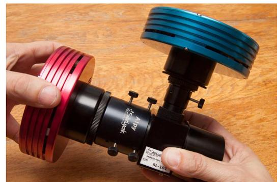
The optimal position is when the vignetting is minimal. When you've found it, tighten firmly the six knurled thumb screws.
